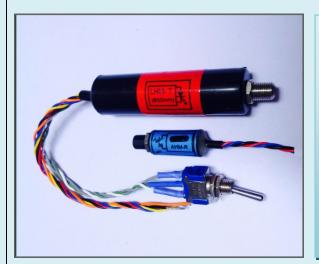
SPECIFICATIONS: LHM-T/650 & AHM-R/RW 650 +/- 5 Wavelength in nm Threshold Current in mA 10 to 15 Optical Power in mW (max) 3 Coupled Power in dBm (max) -3.0 Monitor Photodiode Built-in Analog Bandwidth in Khz Dc to 150 Vin & Vout (Max) in mV 200 & 2000 Modes of Operation APC & ACC Power Supply +6Vdc/100ma Fiber Type PMMA/POF Cable Length 1 to 5 meters Connector SMA Type Rx Gain/ TX Dc Bias Settable as shown below
