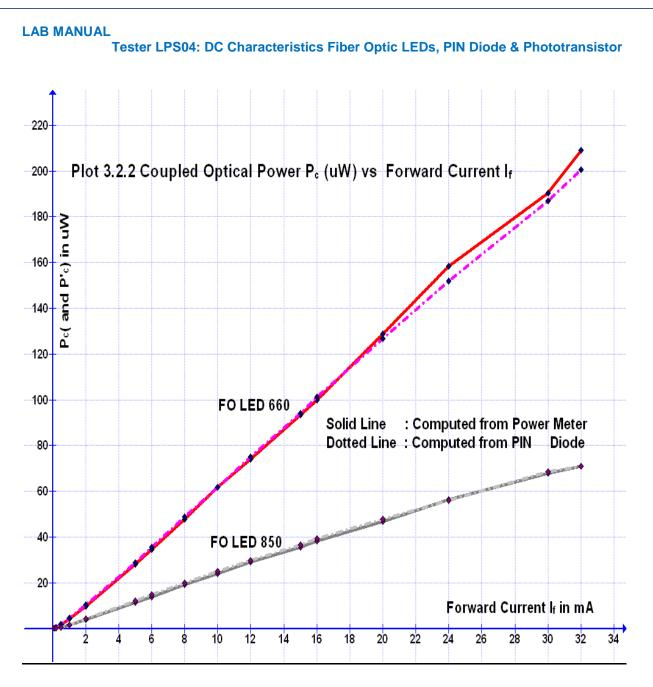
Plot 3.2.2 comprises 4 curves namely,  $P_c$  (uW) and  $P'_c$  (uW) for FO LED 660 and FO LED 850 represented on the linear Y-axis against I<sub>f</sub> represented on the X-axis.
