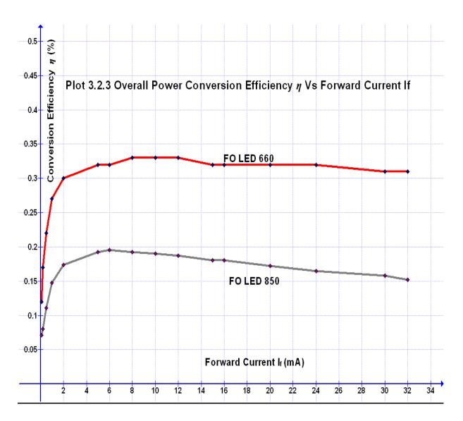
Plot 3.2.3 gives a linear representation of the overall conversion efficiency of optical coupled power as a function of the FO LED forward current.
