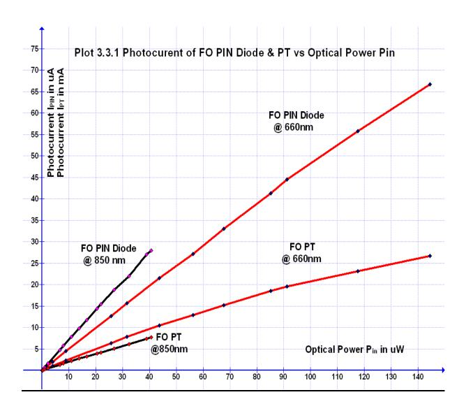
Plot 3.3.1 displays the response of the FO PIN Diode and FP PT to incident optical power at 660nm and 850 nm.
