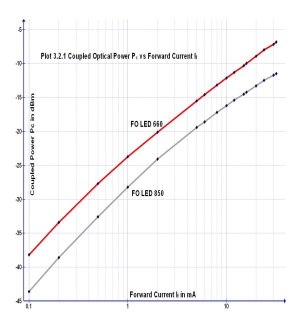
The above is the plot of a typical set of FO LEDs operating at 660nm and 850nm.  $I_f$  is represented on a log X-axis.  $P_c$  (dBm) is on a linear Y-axis. From the graph it is clear that the  $P_c$  varies linearly with  $I_f$  over a wide range in both
