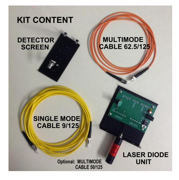
**Tester MCS04: Study of Mode Characteristics of Glass Optical Fibers**
