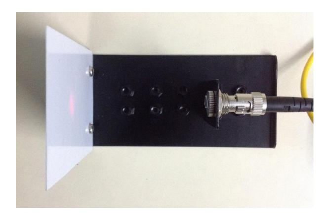
Tester MCS04: Study of Mode Characteristics of Glass Optical Fibers
