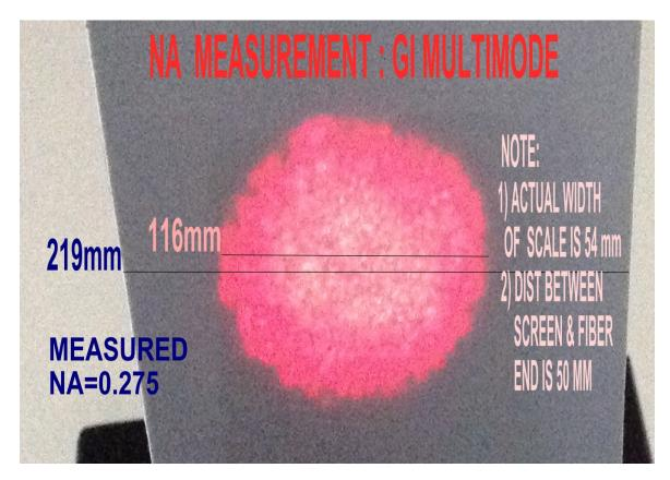
Note: This example refers to a measurement done with 50 mm spacing between screen and the fiber tip
