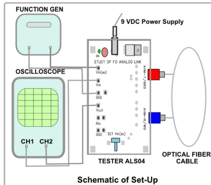
**Optical Fiber Cable** The optical fiber cable links the transmitter to the receiver. The SMA connectors are threaded. While connecting the cable, ensure the threads are in place. Do not apply excessive force on the cup nut.
