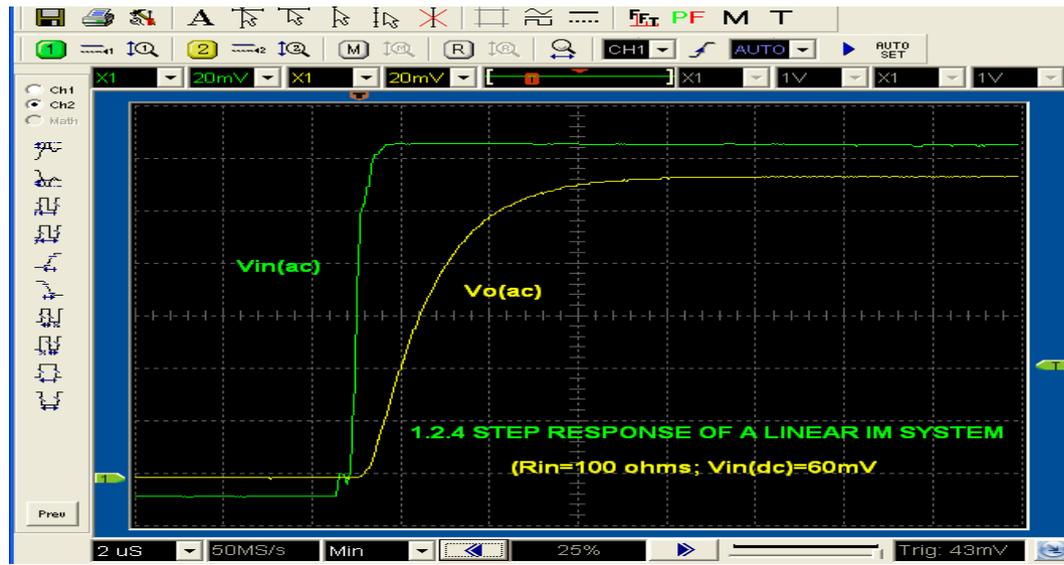
It may be noted that the pulse rise time  $T_r$  is directly proportional to  $R_{in}$ . In applications where speed is not a criteria, the linear modulation system may be used for digital transmission, in conjunction with a comparator.
